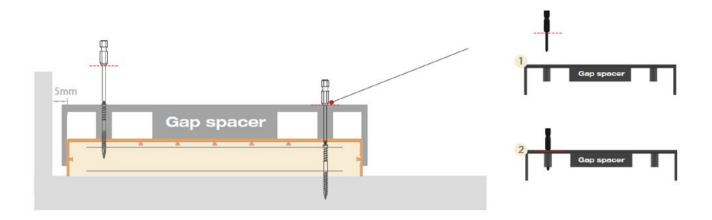
Keep the board 5mm away from the walls or other obstacles to allow for expansion of the composite products and also for ensuring good drainage and ventilation.
